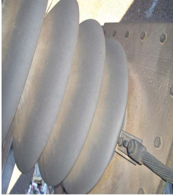
Suppression of leakage current on a coated insulator during slat fog test, the first generation[1]
