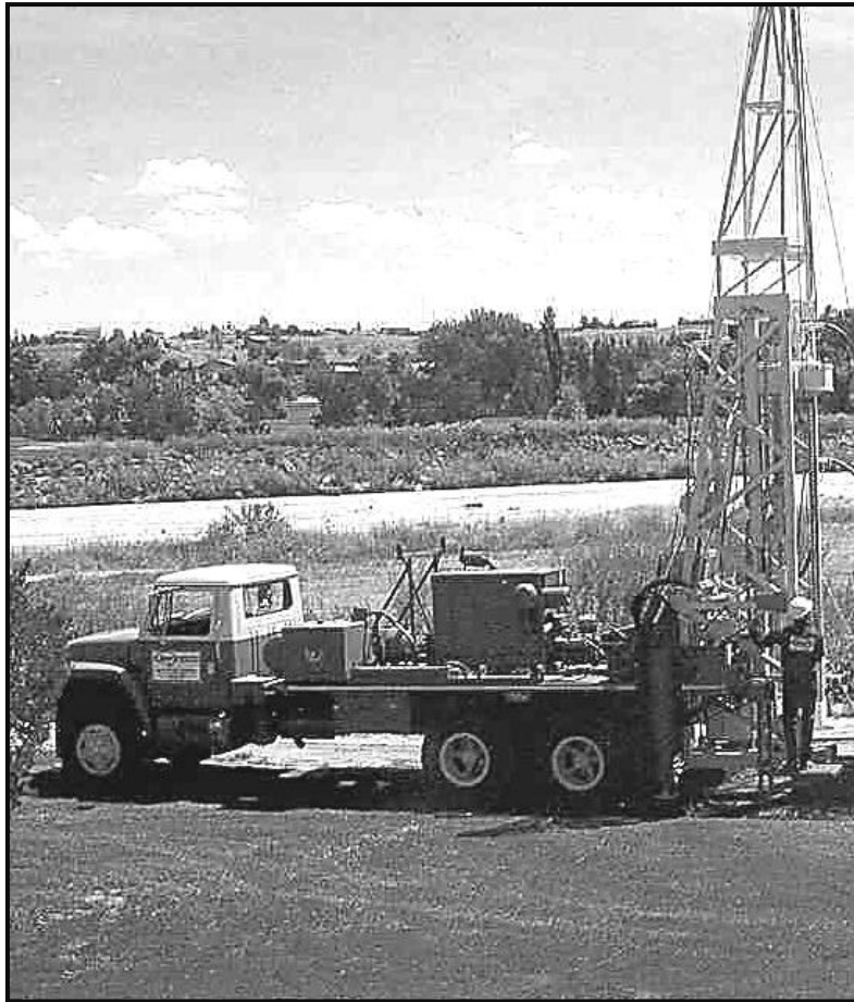
Rotary wash boring
