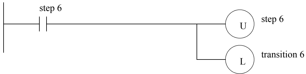
Figure 20.9 SFC Implemented in Ladder Logic
