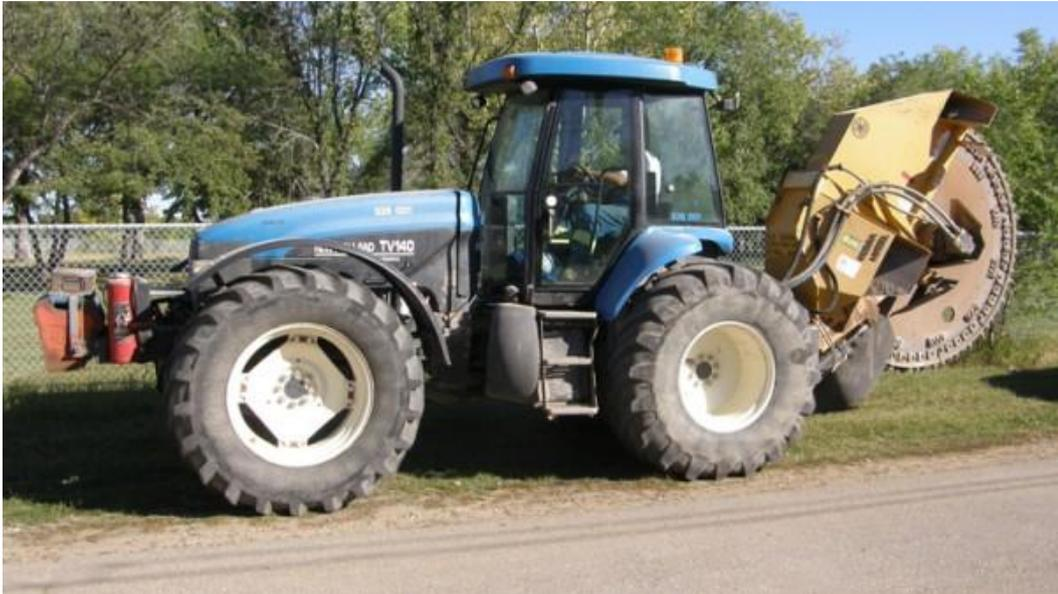
Wheel trencher attached to New Holland tractor
