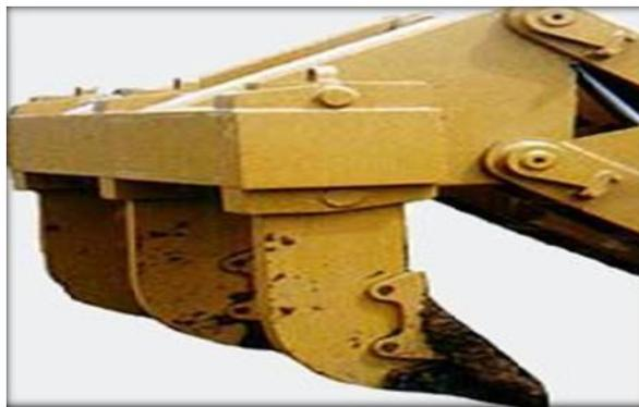
The ripper is the long claw-like device on the back of the bulldozer. Rippers can come as a single shank/giant ripper) or in groups of two or more (multi
