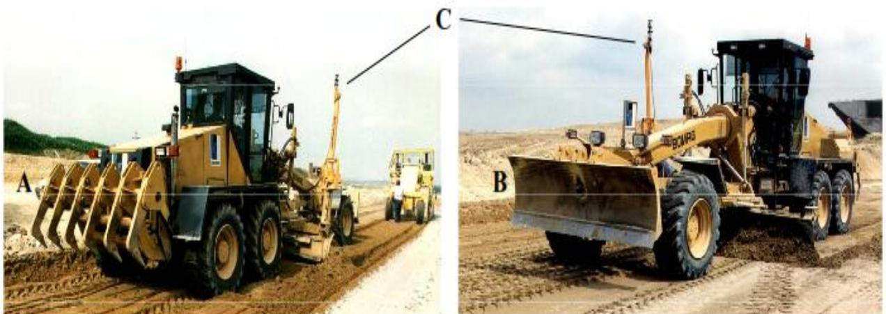
Laser controlled (C) grader equipped with ripper (A) and front blade (B) attachment
