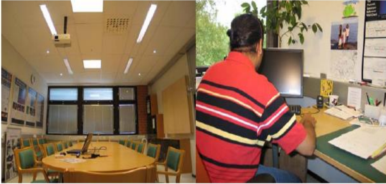
Figure 3-4. Luminaires and windows can induce direct glare, while light reflections from glossy surfaces and computer screens can induce indirect glare.
