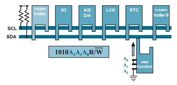
The device that sends data along the bus is called **master**, a device that receives the data is called **slave**. The master starts the transmission with a start signal and stops the transmission with a stop signal on the SDA line. During the start and stop signals the SCL line has to be high. After the master has started the data-transmission with a start signal, the master writes a device address byte to the
