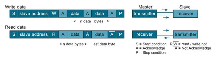
A write operation requires a device address bytes, two address bytes and the data-byte. Upon receive of the address the EEPROM sends an ACK and then clocks in the data-byte. The EEPROM sends again an ACK and the microcontrollers sends a stop-signal to terminate the write sequence.
