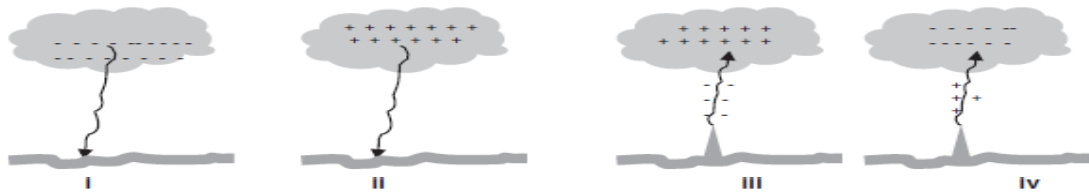
Figure 2.1 (a) Types of cloud flashes: (i) intracloud; (ii) air discharges; (iii) inter-cloud. (b) Types of ground flashes: (i) downward negative ground flashes; (ii) downward positive ground flashes; (iii) upward positive ground flashes; (iv) upward negative ground flashes.
