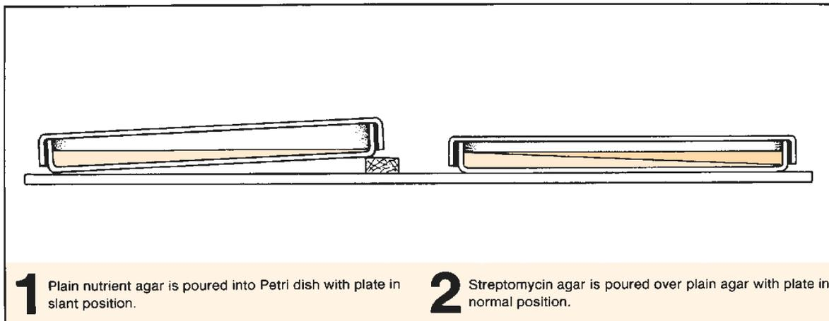
Figure 74.1 Procedure for pouring a gradient plate
