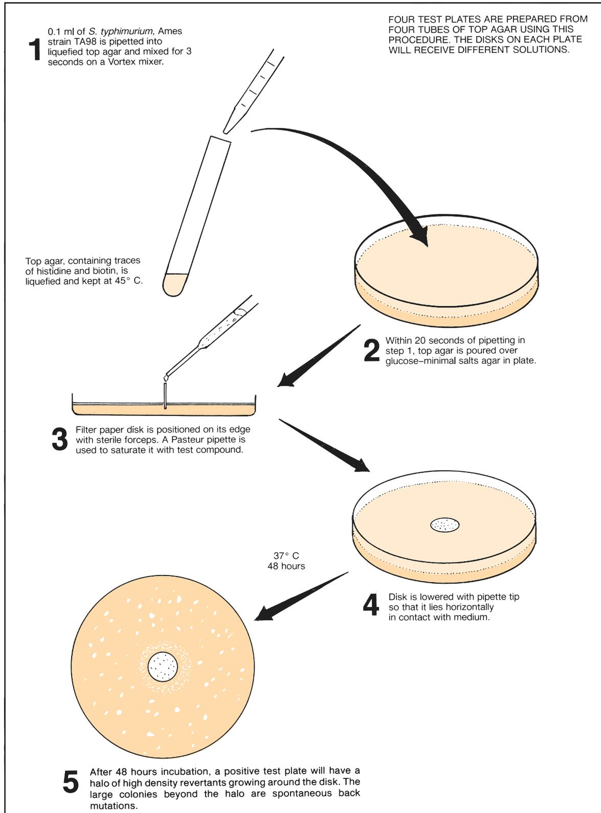
Figure 76.1 Procedure for performing a modified Ames test
