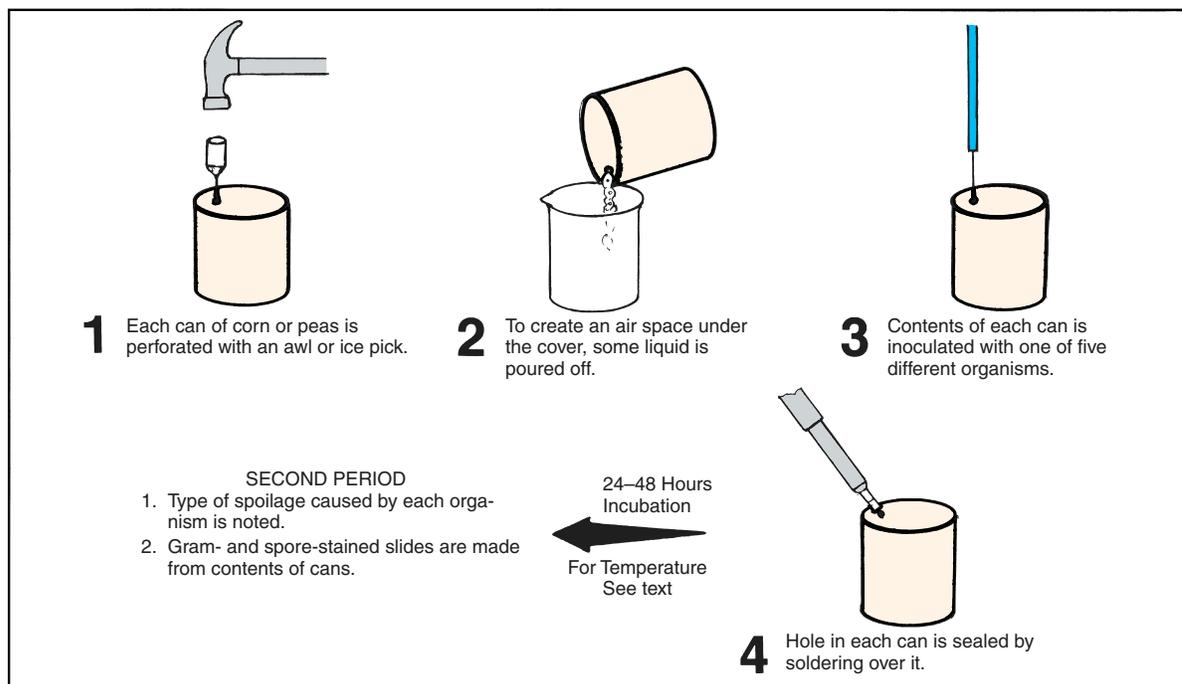
Figure 70.1 Canned food inoculation procedure
