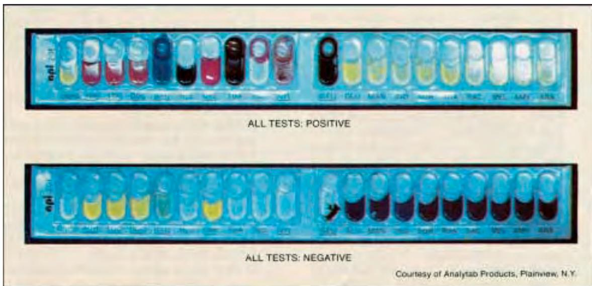
Figure 52.1 Positive and negative test results on API 20E test strips
