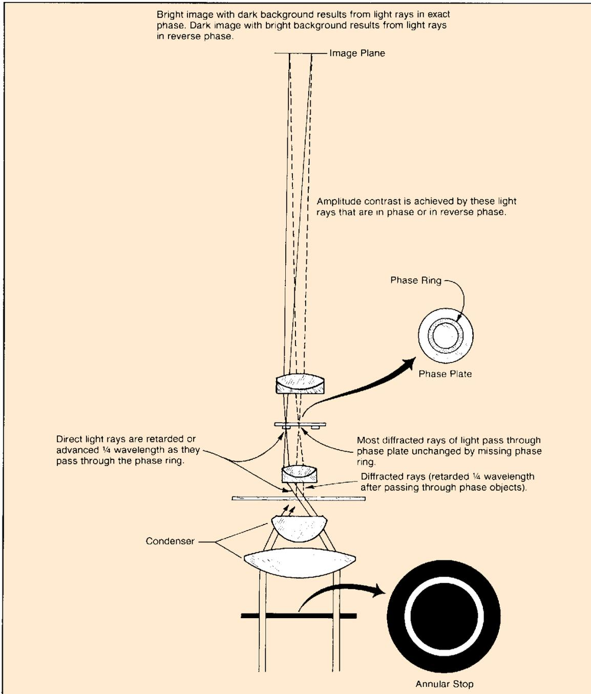
Figure 3.3 The optical system of a phase-contrast microscope
