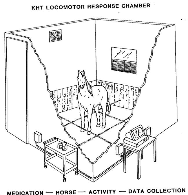
**Fig. 1.** Schematic diagram of behaviour chamber with infrared sensors spaced around the stall to measure activity.
